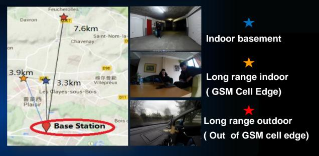
Coverage Gain(NB vs GSM)
