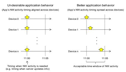
Figure 7: Spreading an Application's Network activity timing within an acceptable window
