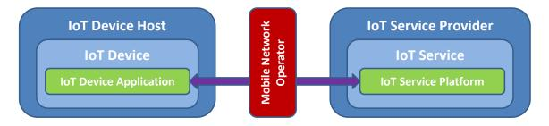
Figure 2: Generalised IoT Service Architecture
