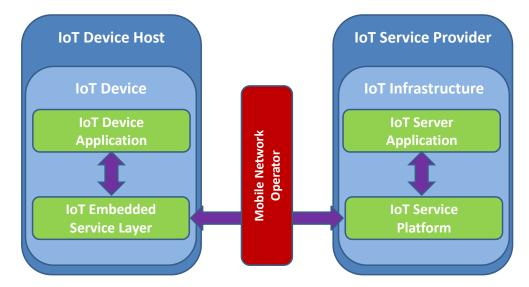
Figure 3: Generalised "Layered" IoT Service Architecture
