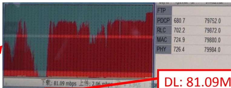
Snapshot of TD-LTE peak throughput test
