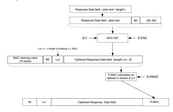
Figure 34: TLV Response Data Field Encryption
