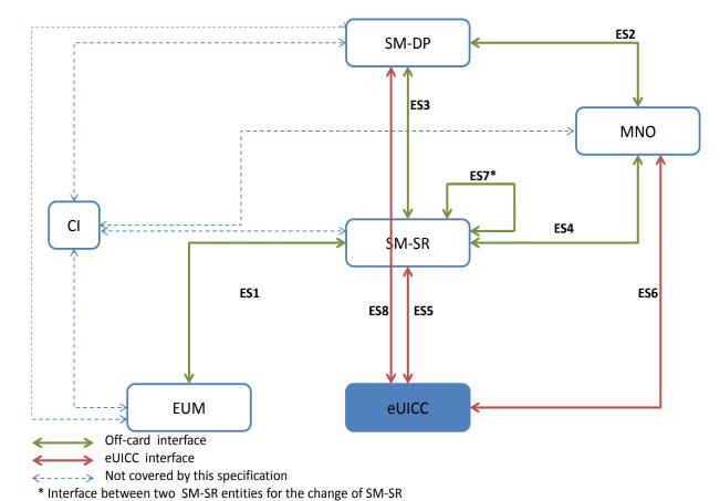
Figure 1: eUICC Remote Provisioning System
