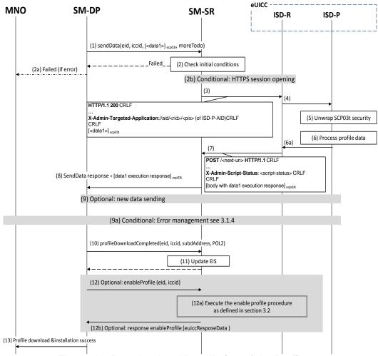
Figure 12: Download and Installation of the Profile
