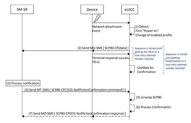
Figure 29: Sequence Flow of Notification Over SMS
