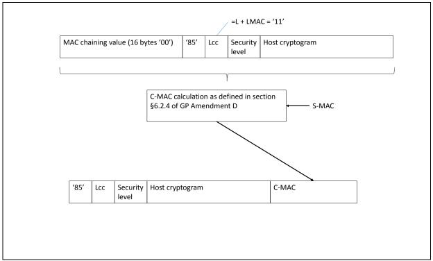
Figure 32: TLV Command Data Field Encryption
