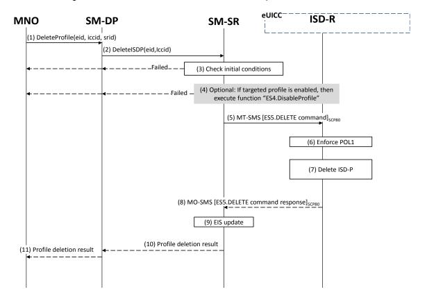
Figure 21: Profile and ISD-P Deletion via SM-DP
