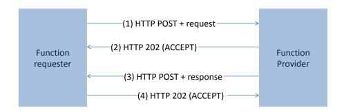
Figure 142: MEP: Asynchronous Request-Response With Callback
