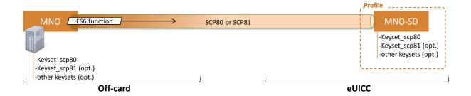
Figure 7: Secure Channel Between MNO and MNO-SD
