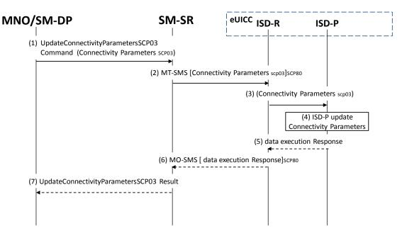
Figure 28: Connectivity Parameters Update Using SCP03
