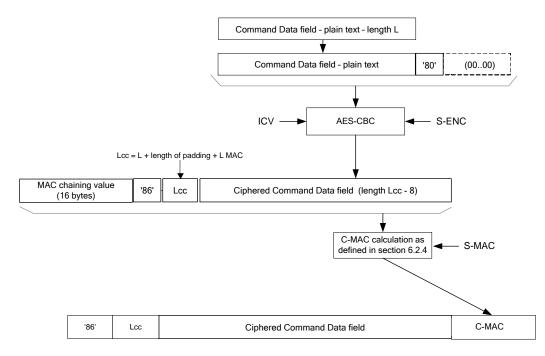
Figure 33: TLV Command Data Field Encryption
