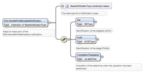
Figure 131: <rps:ES4-HandleProfileEnabledNotification>
