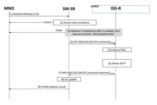
Figure 20: Profile and ISD-P Deletion
