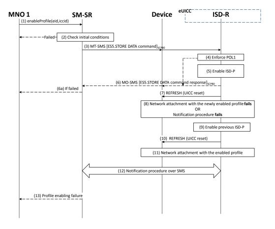
Figure 15: Profile Enabling failure, with roll-back
