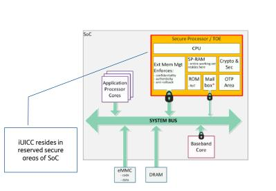
New HW-based non-standardized eUICC form factor . This can operate complementary to GSMA Remote SIM Provisioning. It may also increases SIM performance and available memory. Functional, security and certification aspects will be demonstrated in the PoC
