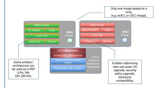
The MNO remains in control of the entire image (as of today) that can be a GSMA Remote SIM Provisioning (eUICC) image and can evolve over time (future-proofness).
