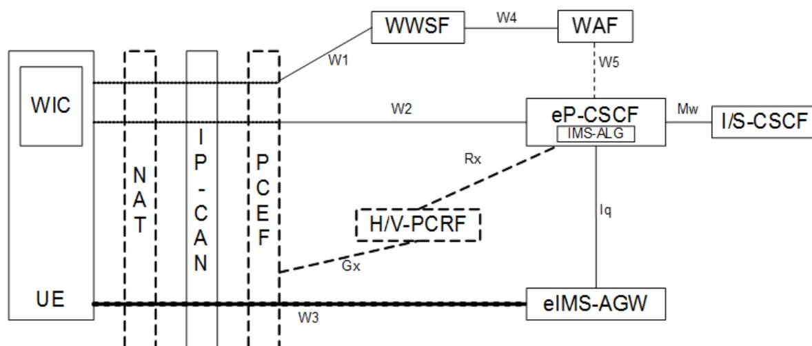
**Figure 6: WebRTC reference architecture to IMS and reference model (3GPP TR 23.228)**
