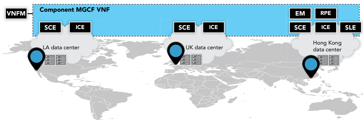
Figure 7 – An MGCF VNF with decomposed functionality can spin up VNFC instances of specific resources where and when they are needed to provide more efficient performance.
