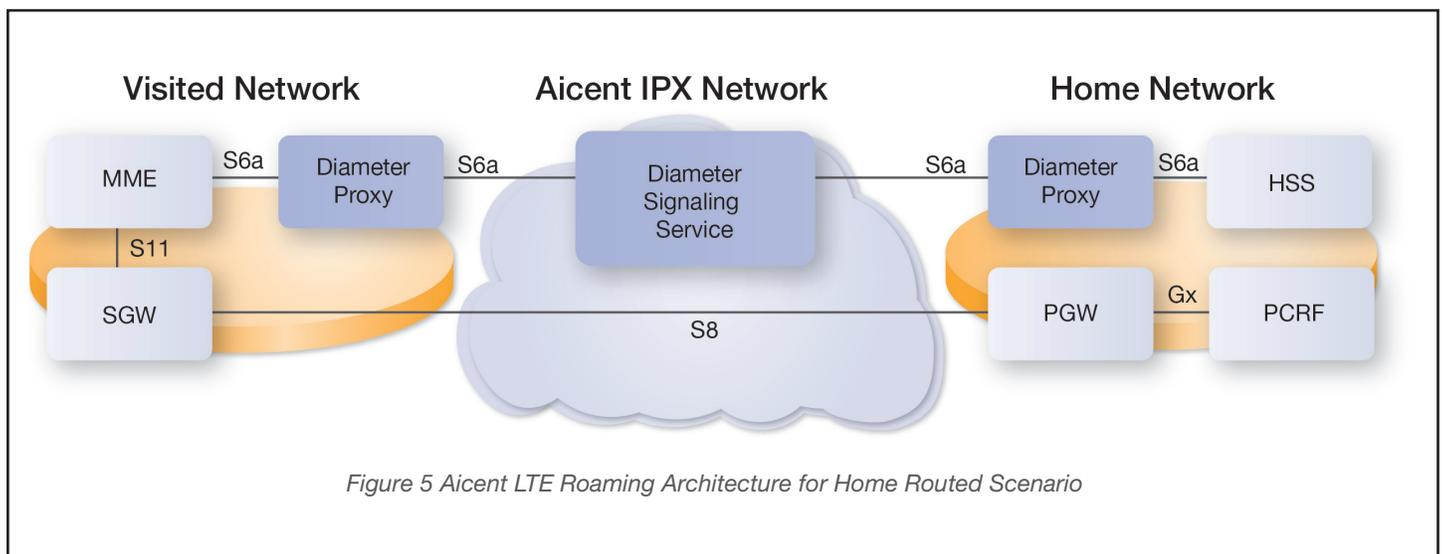
Figure 5 Aicent LTE Roaming Architecture for Home Routed Scenario
