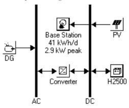
The technical dimensioning proposed for Banglalink contained detail site and model wise data. An example is as follows:
