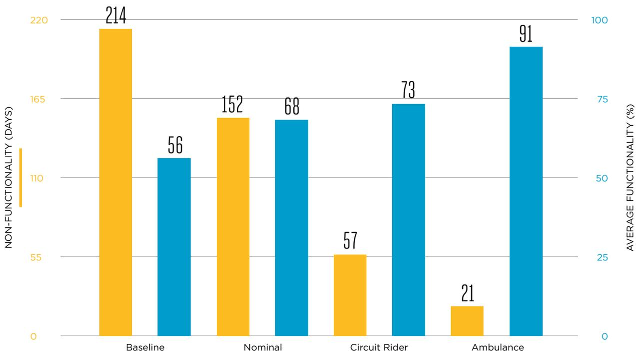
**Sensor-driven ambulance maintenance results in a significantly higher proportion of functional days<sup>24</sup> than other models.** Handpumps serviced by the ambulance model were functional nearly 91 per cent of the time, which was a statistically significant<sup>25</sup> difference
