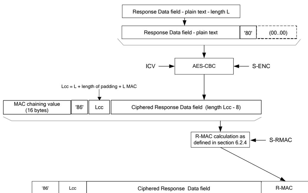
**Figure 34: TLV Response Data Field Encryption**
