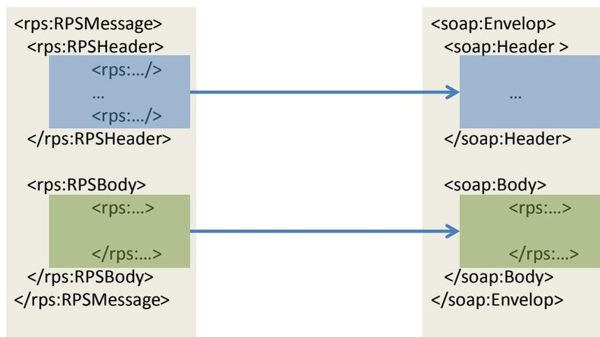
Figure 140: RPS Message Binding
