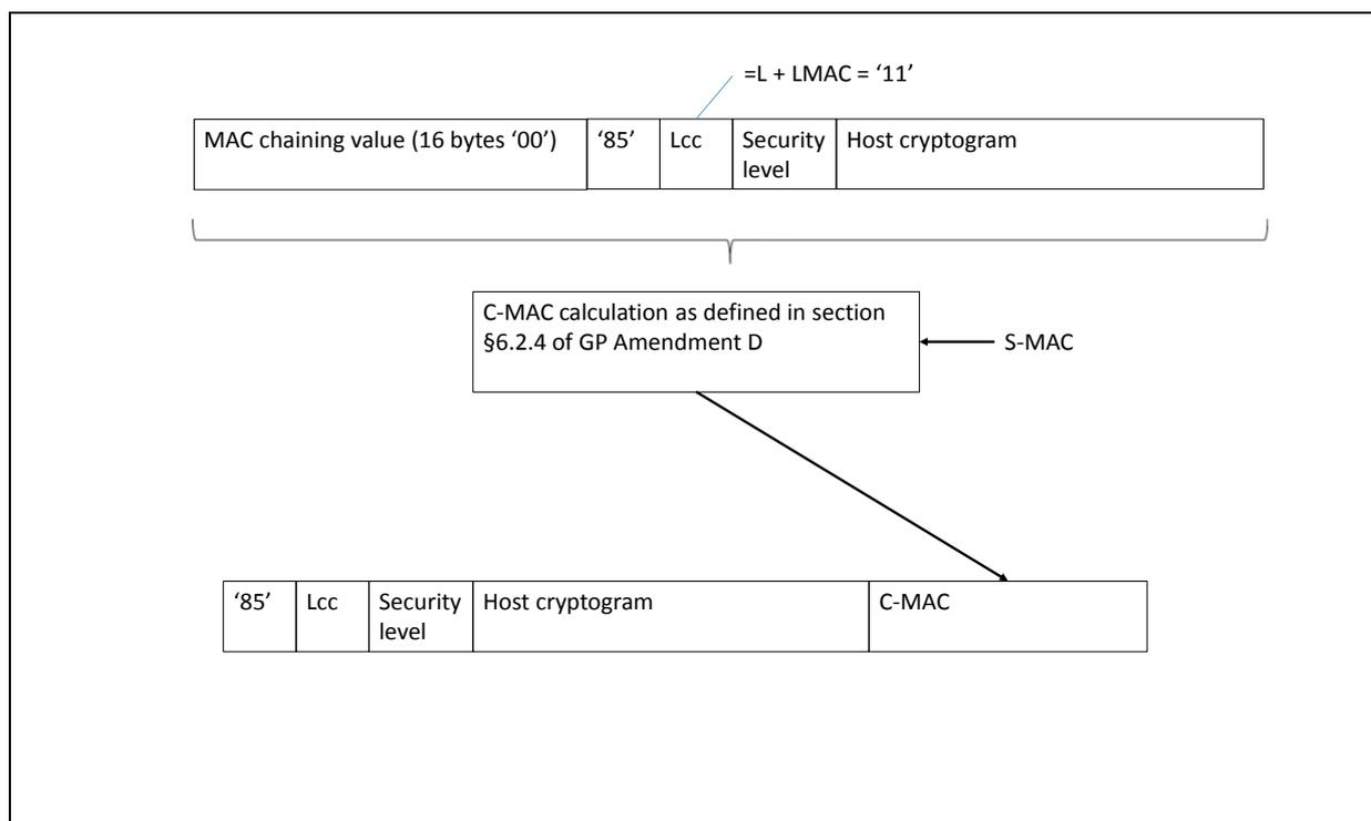
**Figure 32: TLV Command Data Field Encryption**
