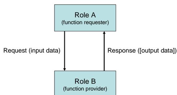
**Figure 35: Functions as a Request-Response Data Exchange**
