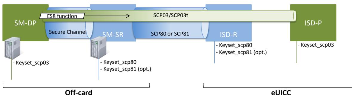
Figure 6: Secure Channel Between SM-DP and ISD-P
