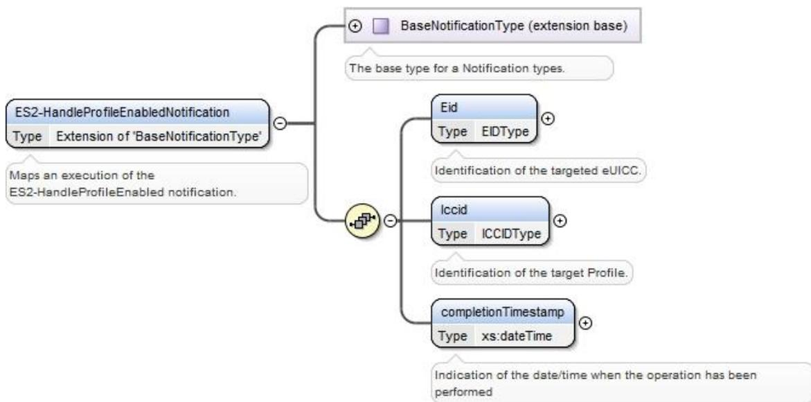
**Figure 83: < rps:ES2-HandleProfileEnabledNotification >**
