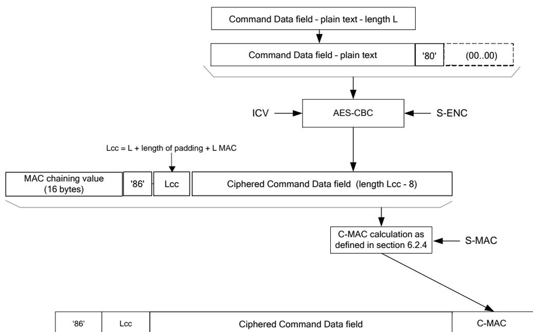
**Figure 33: TLV Command Data Field Encryption**
