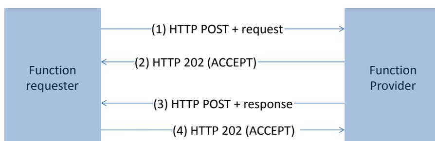
Figure 142: MEP: Asynchronous Request-Response With Callback
