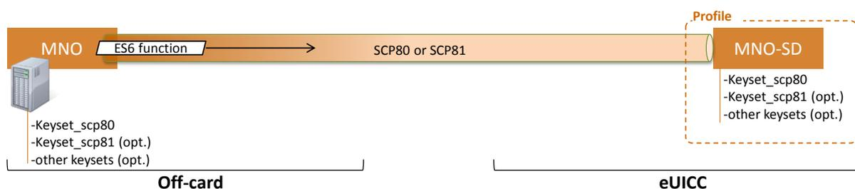
Figure 7: Secure Channel Between MNO and MNO-SD
