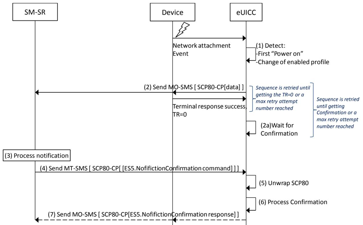
**Figure 29: Sequence Flow of Notification Over SMS**
