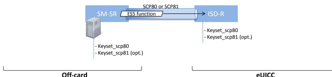
**Figure 5: Secure Channel Between SM-SR and ISD-R**
