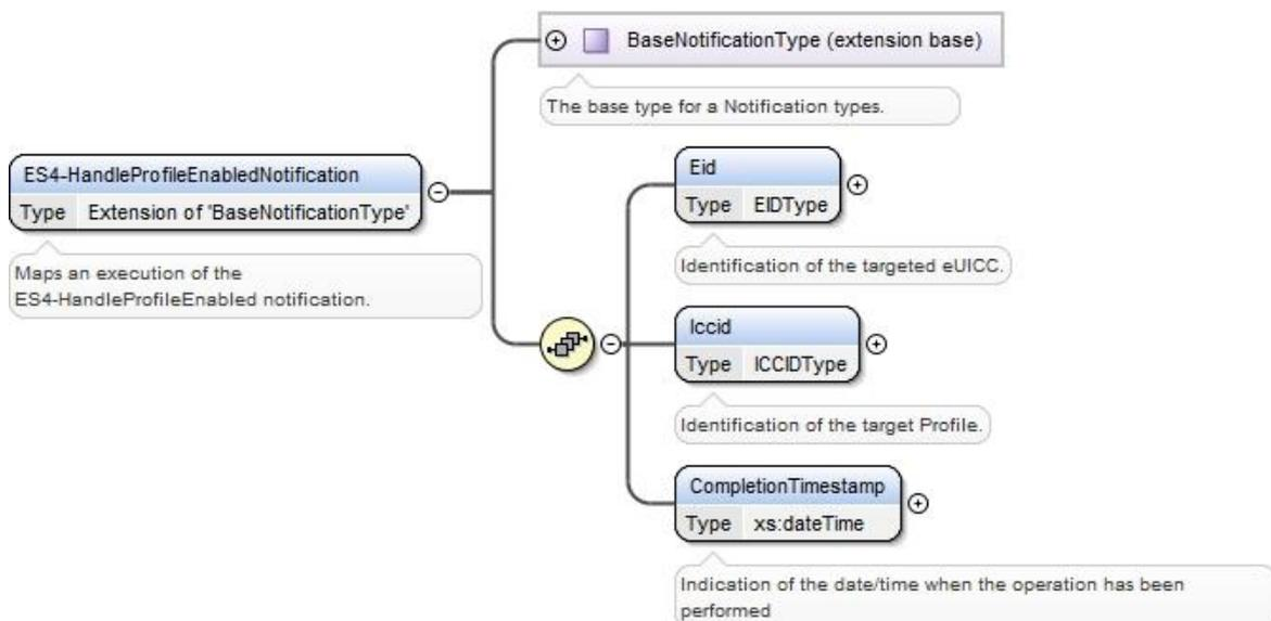
**Figure 131: <rps:ES4-HandleProfileEnabledNotification>**
