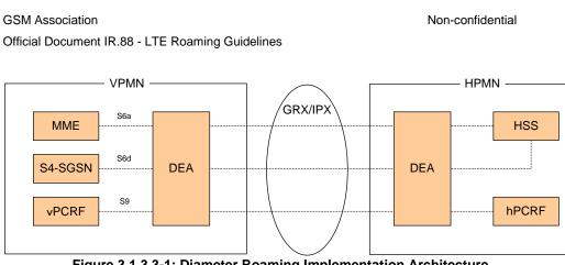
Figure 3.1.3.3-1: Diameter Roaming Implementation Architecture
