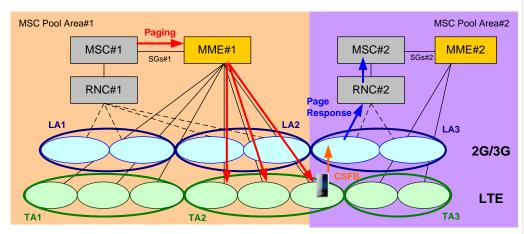
Figure 5.2.1.2-1: CSFB issue due to TA/LA misalignment
