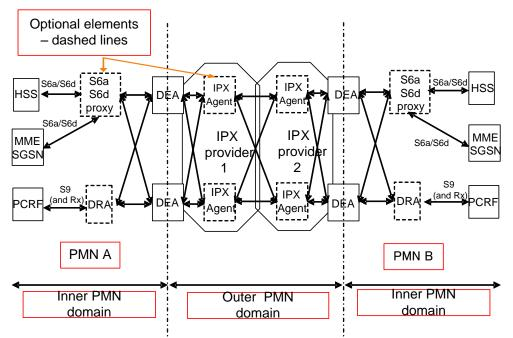
Figure 3.1.3.3-2: End to end Diameter Architecture
