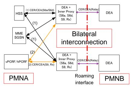
Figure B-2: Diameter architecture example 2
