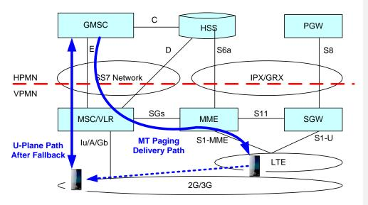
Figure 5.2.1.1-1: CSFB Roaming Architecture
