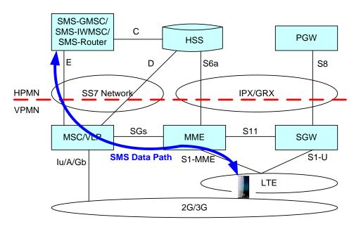
Figure 5.1.1-1: SMS over SGs Roaming Architecture
