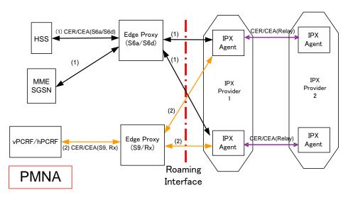
Figure B-5: Diameter architecture example 5
