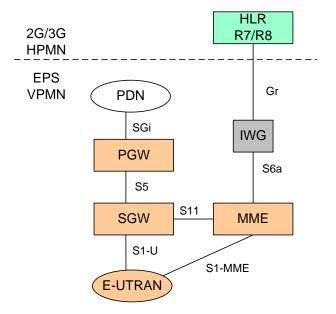
Figure 4.1.3-1: HPMN Legacy Roaming Architecture (local break-out)
