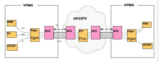
Figure 6.5.1-3: Security for IPX Service Hub connectivity
