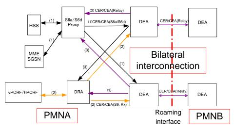
Figure B-1: Diameter architecture example 1
