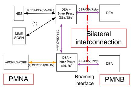
Figure B-3: Diameter architecture example 3
