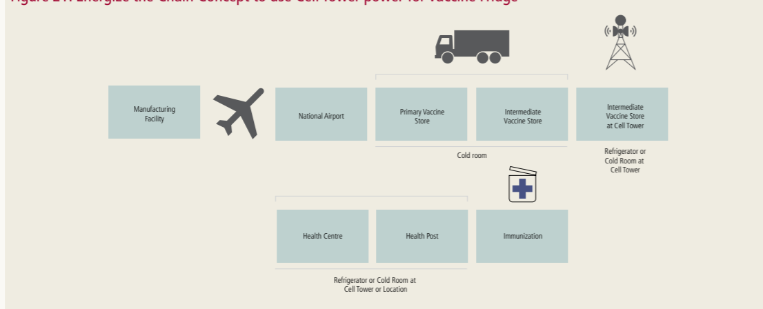
Figure 21. Energize the Chain Concept to use Cell Tower power for Vaccine Fridge
