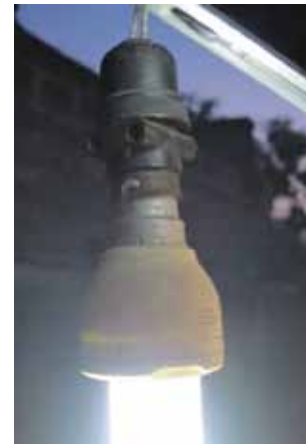
Husk Power customers can charge their phones via a power socket in the light fittings
