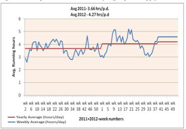
The above graph shows that the usage of diesel generator has increased from an average of 3.66 hours/day in 2011 to 4.27 hours/day in 2012. This increased dependence on diesel generator can be attributed to reduced availability of grid power supply and to the deterioration in the quality of grid power supply.
