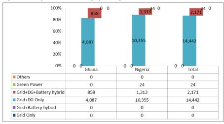
Figure 8: Sites by Power Solution Deployed (on-grid)<sup>11</sup>
