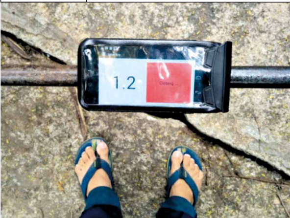
ValveKey app for a valve turned 1.2 rotations and being closed
