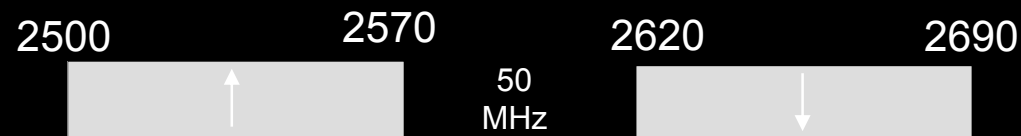
The 2600 band: 2X70 MHz and 50 MHz unpaired
