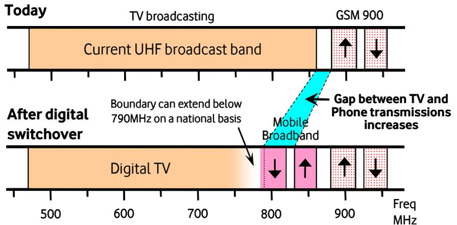
The downlink transmissions from the mobile network will come from basestation antennas at the top of a mast. This is similar to the configuration of a broadcast network, so the interference to TV sets from mobile transmitters is unlikely to be substantially different to broadcasting. Advances in technology make it possible for these transmissions to spill less into neighbouring channels (i.e. the broadcast spectrum) than for the existing mobile bands.
