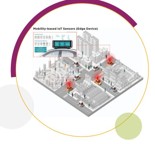
check data from multiple taxis to ensure the information it is collecting from the sensors is accurate: Frequent changes in the temperature and humidity can require individual sensors to be recalibrated.
