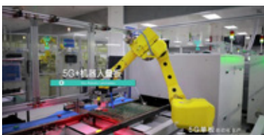
Assistance of 5G + cloud-based machine vision in the precise positioning for robotic arm lamination
