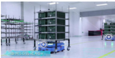
Jack-up 5G-powered AGVs operating in the SBC area
