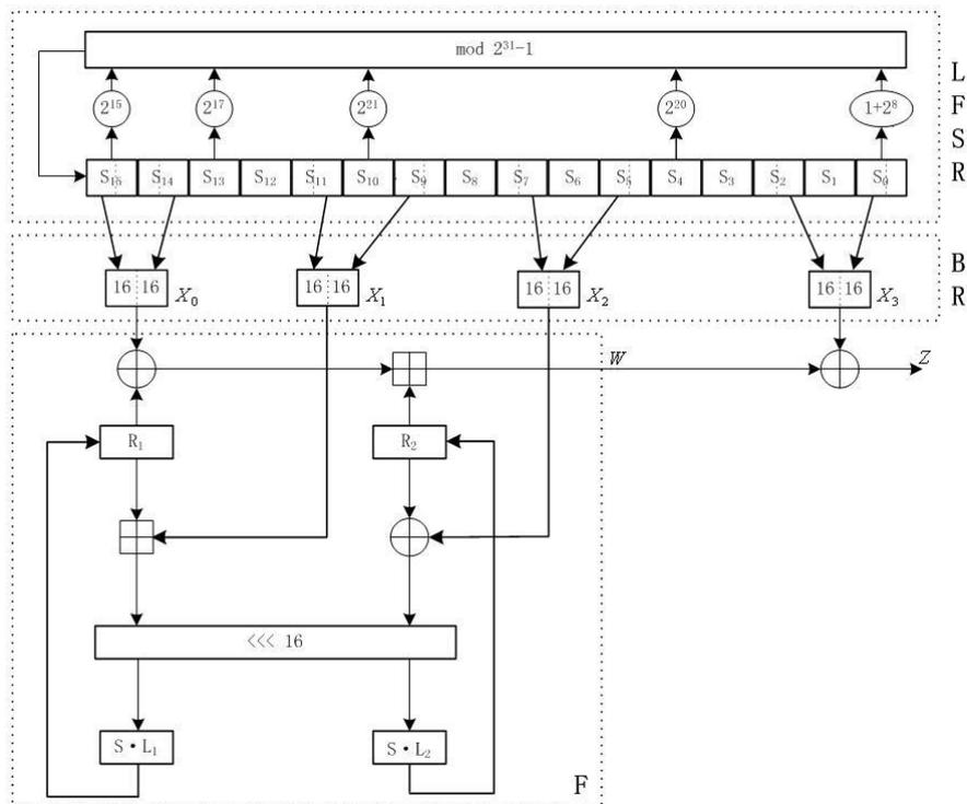
**Figure 8.1: The structure of ZUC**
