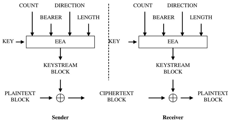
**Figure 7.1: Ciphering of data**
