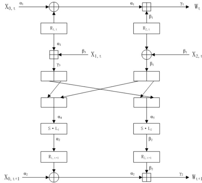
**Figure 12.1: The linear approximation of two-round  $F$**
