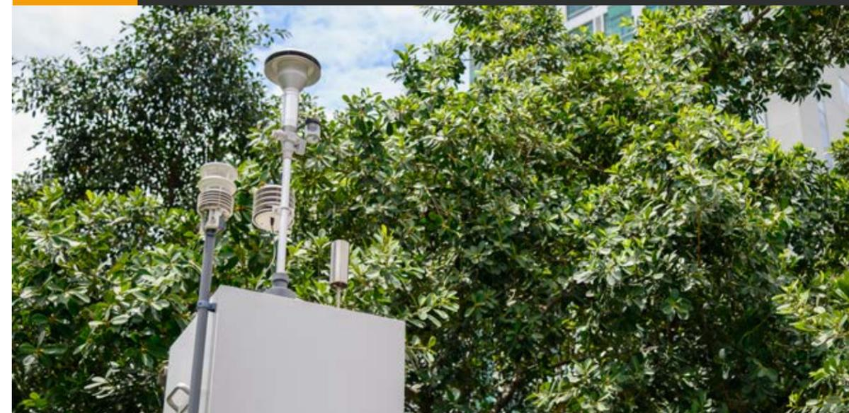
Deutsche Telekom and sensor provider Smart Sense have developed and deployed Smart AirQ monitoring system – a smart sensor platform for monitoring air quality – in Croatia, Germany, Greece and Saudi Arabia. The system supports indoor and outdoor monitoring of multiple air quality parameters at room, street and city level including relative humidity, temperature, atmospheric pressure, CO<sub>2</sub>, NO<sub>2</sub>, NO<sub>x</sub>, CO, SO<sub>2</sub>, O<sub>3</sub> and airborne particles.
