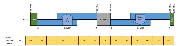
Figure 24 APT frequency arrangements and an 8 MHz TV channel raster in the 700 MHz band
