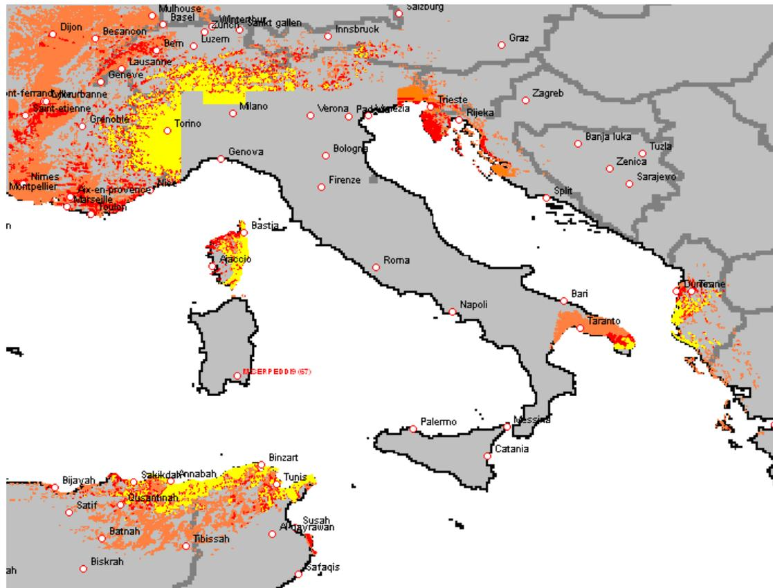
Figure 19 Cumulative interference on channel 68
