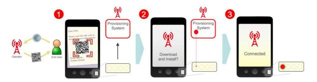
Remote SIM Provisioning Operation – Operator Profile Installation
