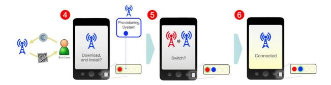
Remote SIM Provisioning Operation – Operator Profile Selection
