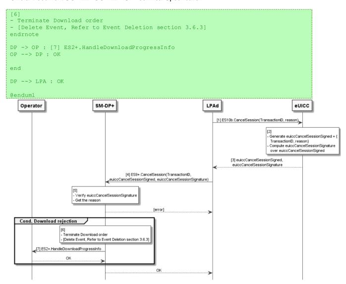
Figure 12: Sub-procedure Profile Download and Installation - Download Rejection
