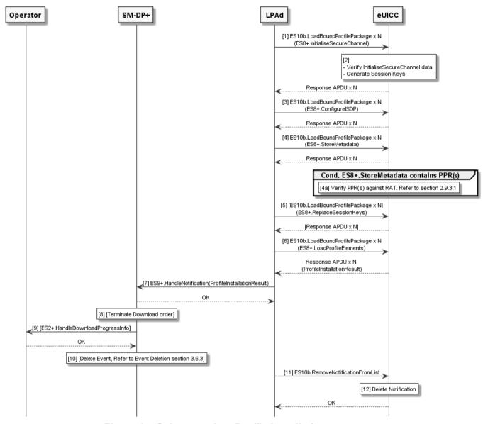
Figure 14: Sub-procedure Profile Installation
