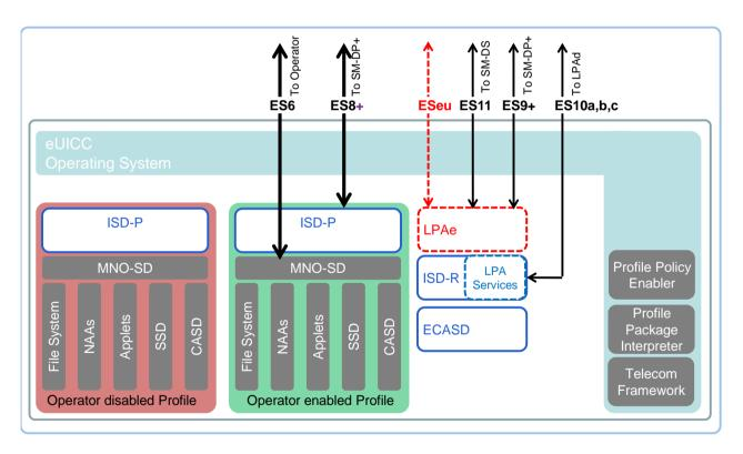
Figure 3: Schematic Representation of the eUICC
