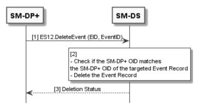
Figure 28: Event Deletion Procedure without Cascade
