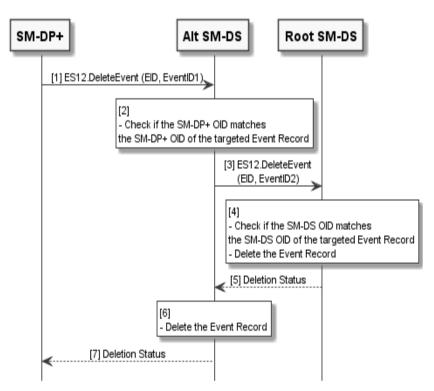
Figure 29: Event Deletion Procedure with Cascade
