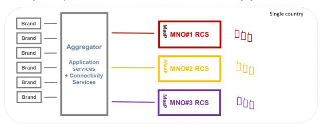
its own network enabled for RCS (via its IMS and an RCS AS, see previous chapter) and it runs its own MaaP instance, which offers interfaces to Aggregators. With this setup the RBM services are offered under the T&Cs of the MNO.
