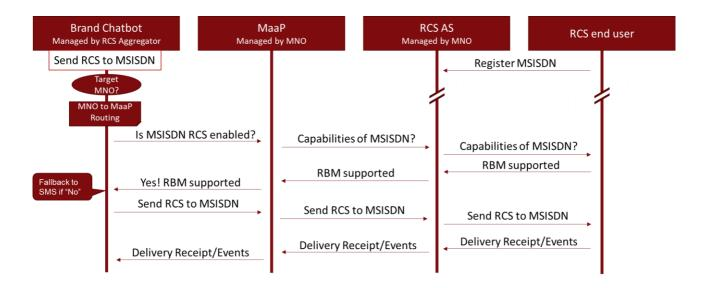
Now, the actual RCS communication can commence: Asking the MaaP about the RCS capability of the specific MSISDN (in order to determine if an SMS fallback is needed). After these enquiries, the RCS message can be submitted to the MaaP instance. The MaaP instance then hands the message over to the IMS with its RCS AS, which eventually delivers it to the end user.
