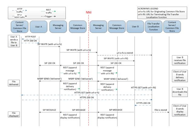
Figure 18: File Transfer Localisation Function: global flow
