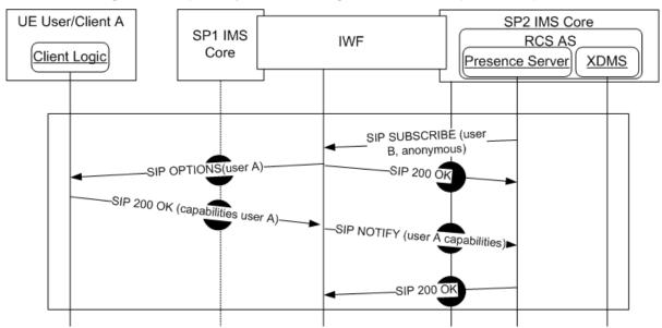
Figure 5: Capability interworking via network: Presence request
