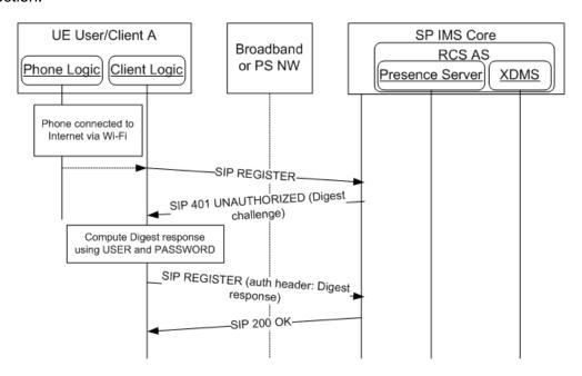
Figure 7: Registration with SIP Digest Authentication
