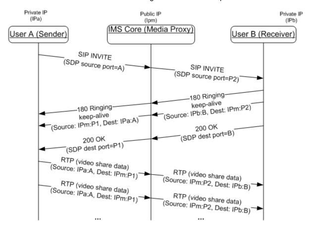
Figure 6: RTP symmetric media path establishment
