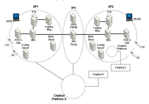
Figure 1: Simplified Example of RCS Architecture
