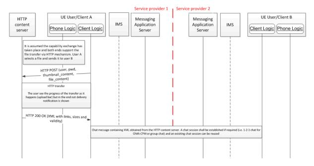
Figure 8: File Transfer: Sender procedures
