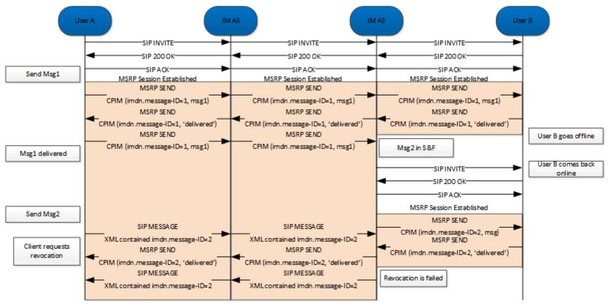
Figure 34: Message Revoke, Failed request\*
