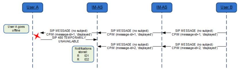
Figure 31: Store and forward: Message(s) displayed notifications via SIP MESSAGE with sender offline\*
