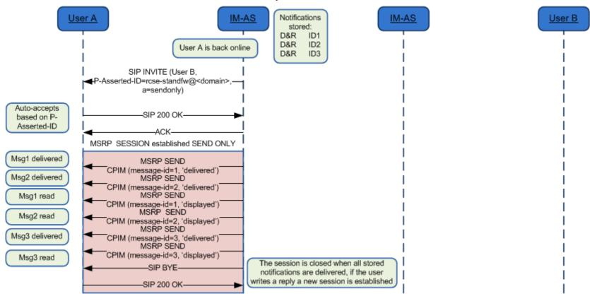
Figure 30: Store and forward: Notification(s) deferred delivery\*
