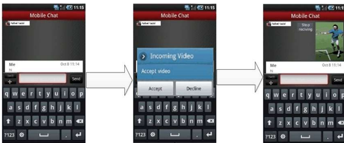
Figure 107: Reference UX for accessing Video Share without a call for the receiving side during a chat
