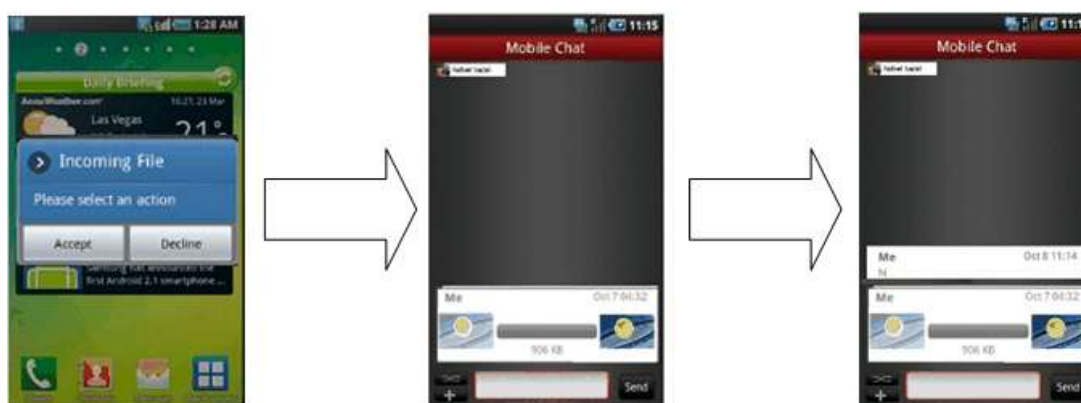
Figure 47: Reference UX for File Transfer on the receiver side
