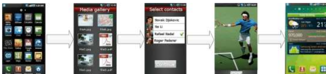
Figure 102: Reference UX for accessing Video Share without a call from media gallery
