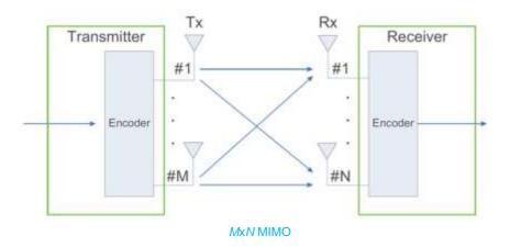
In the early phase of LTE, 2x2 MIMO was the predominant technology. With the increase of network capacity and experience requirements, especially the popularization of four-antenna terminals, operators have begun to substantially deploy the four-antenna technologies. Currently, four-antenna technologies have been deployed on 180 networks worldwide.
