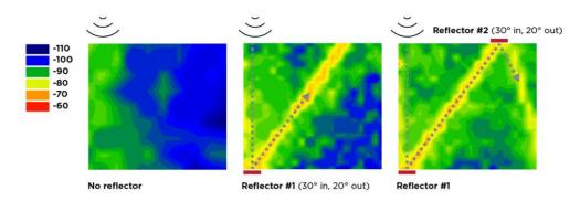
• Enhancement – A design antenna pattern is used as an enhancement "lens" to refocus the signal to a certain direction. Ideally, the lens would be installed on the door or windows, which would then boost an incoming signal into the entire room. The signal strength could increase more than 10 dB, as shown by the radiation pattern after applying the lens in Figure 16.
