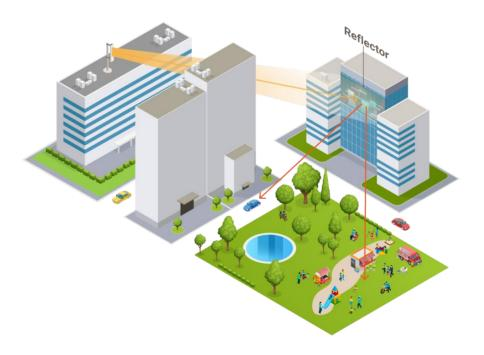
An outdoor NLOS deployment scenario is shown in Figure 13. The signal from the gNB is blocked by tall buildings. By integrating an RIS within the advertising display, the street, park area and walkway could be well covered through the signal redirection. The same deployment scenario could also be applied to stadiums and public squares that are equipped with a large display, and also for office buildings in which a RIS can be integrated into the glass exterior.
