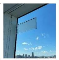
Internal CPE antenna provides the best customer self-install option. Smartphone applications can find the best position in the home, usually near a window on the best coverage side of the house. However, there may be aesthetic considerations for the position or location of the CPE.
