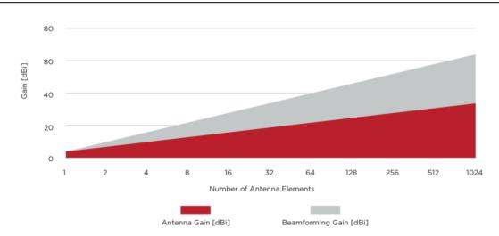
Figure 7: mWave theoretical Antenna and Beamforming gains
