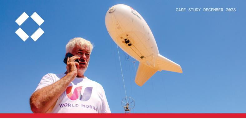
However, Gregory Gottlieb estimates that each additional radio would add about 20 kg to the payload of the aerostat. As one cubic metre of helium is required to lift 1 kg, adding new radios would increase the helium required, as well as the power consumed by the aerial base station.
