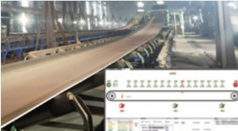
Sealing-tape machines are prone to motor or reducer failures, belt misalignments, slip, tearing, and other issues during production and operation due to the complex operating environment, the long transportation distance, and the large transportation volume. What's worse, the lack of effective detection and monitoring methods can lead to consequences ranging from lowered production efficiency to severe accidents.
