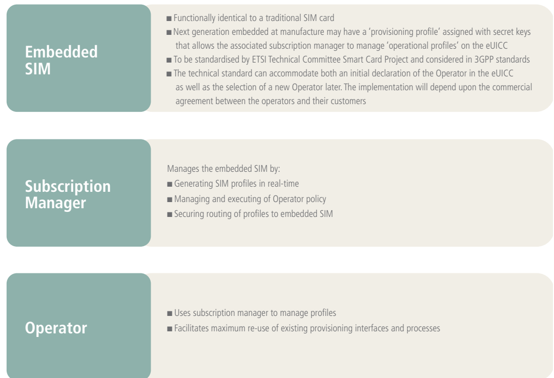
Figure 11. Remote Provisioned SIM: Roles
