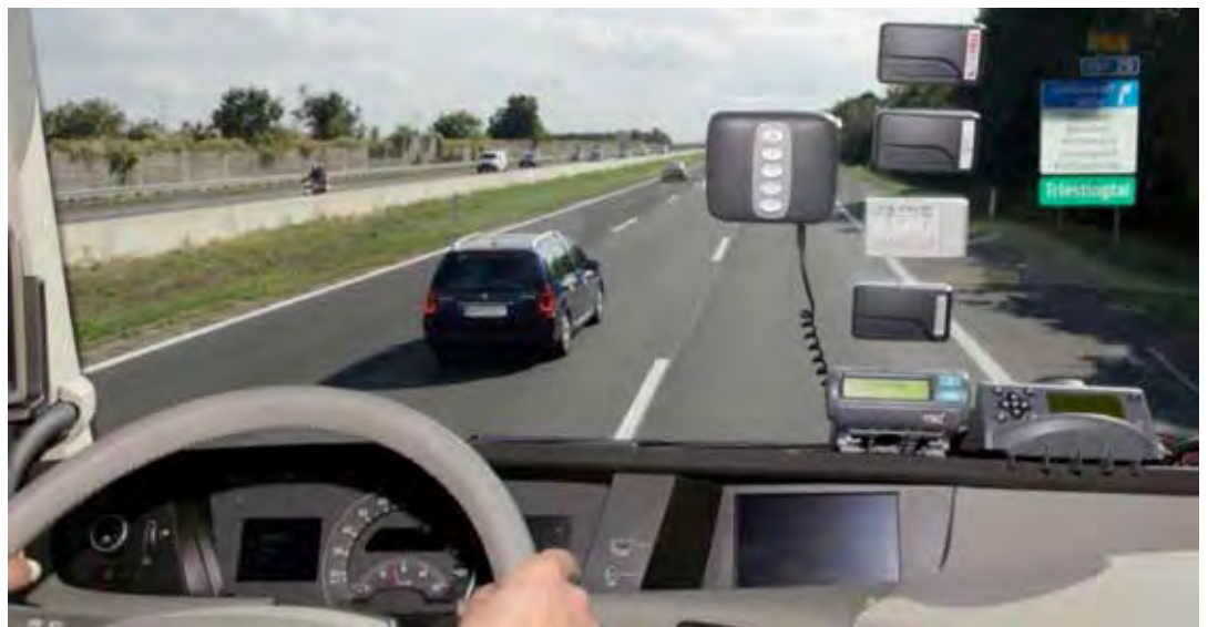
FIGURE 6: THE WINDSHIELD OF A TOLL-COMPLIANT TRUCK TODAY
