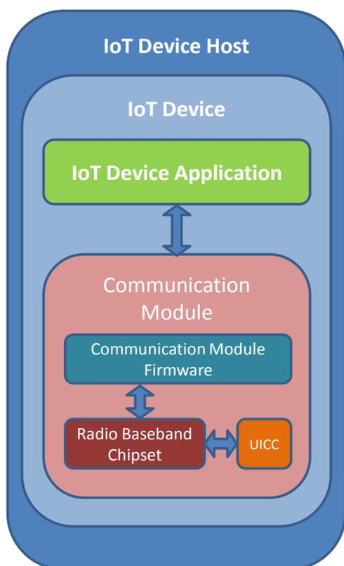
**IoT Device Host** – The application specific environment containing the IoT Device e.g. vehicle, utility meter, security alarm etc.
