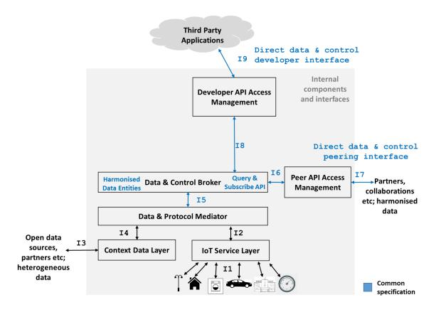
Figure 2: Architecture for offering only Direct Data/ Control Services
