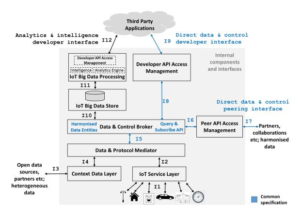
Figure 5: General architecture for fully scoped IoT Big Data
