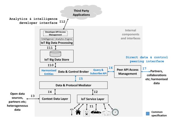
Figure 4: Architecture for offering Analytics & Intelligence over Harmonised Sources
