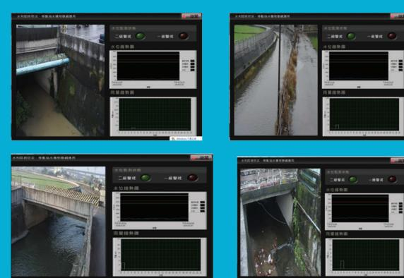
Real time monitoring of water levels via LTE communications
