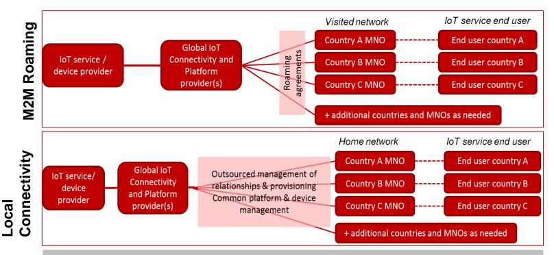
Hybrids models of M2M roaming and local connectivity could also be deployed, and new models might emerge in future
