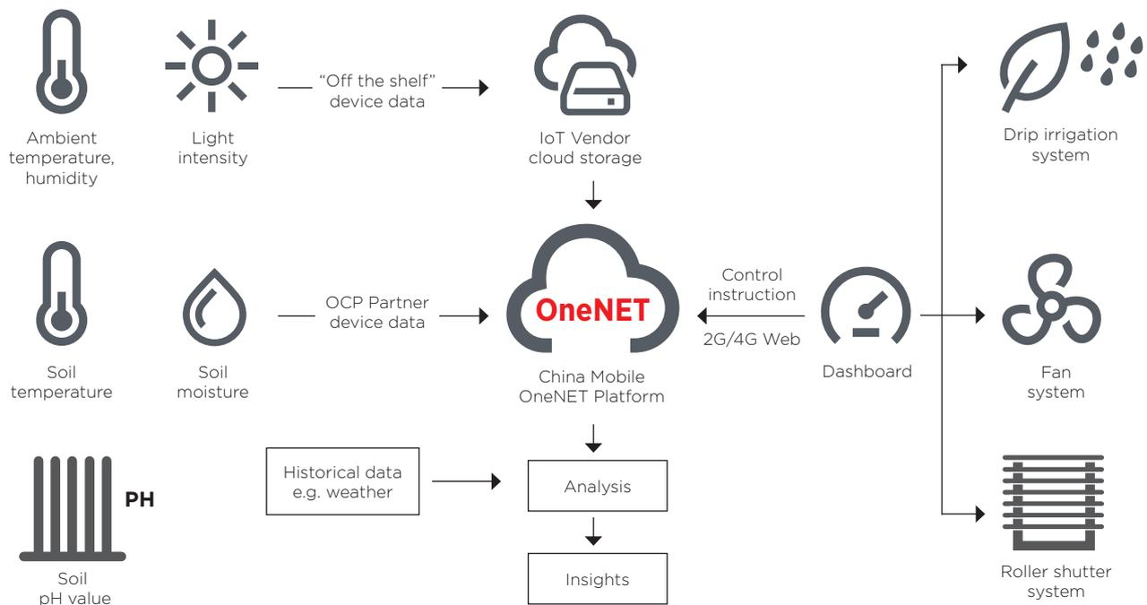
**Figure 6** The OneNET Platform aggregates data from OCP partner devices and from “off the shelf” device vendor cloud services and manages access to the stored data by integrated smart hardware solutions (such as irrigation) and analytic applications.
