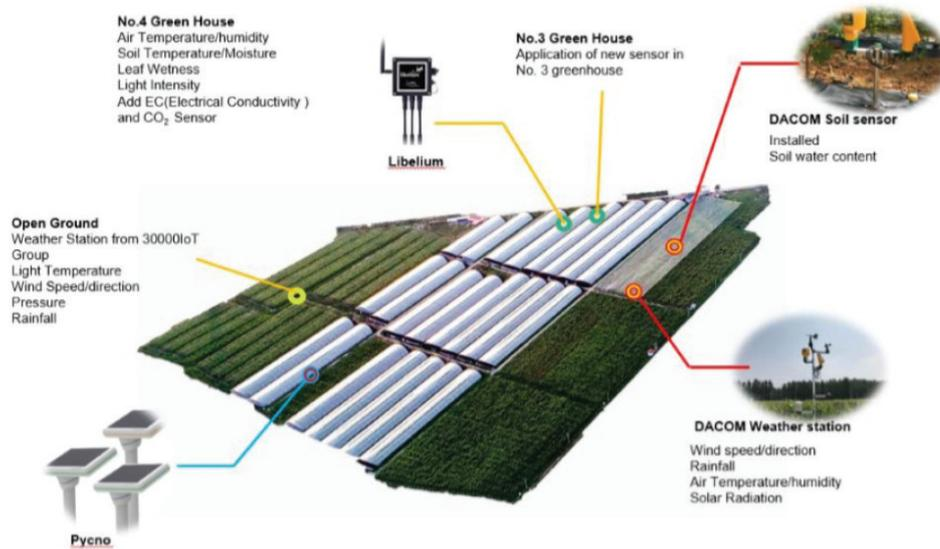
A ‘connected’ weather station has also been deployed to obtain more accurate environmental data at the location and support “intelligent” irrigation. Various additional devices provide air pressure meters, soil moisture sensors, irrigation controllers, solenoid valves, switches, and smart water meters.
