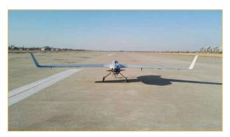
Figure 1 Hybrid wing high-altitude long-endurance UAV
