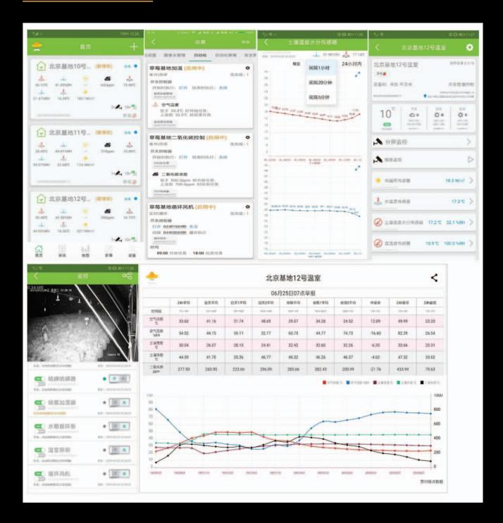
The LinkDotter Butler application enables the producer to monitor the greenhouse environment, view the status of, and data recorded from, individual sensors and set automatic controls for the management devices to adjust the environment. For example when the substrate moisture level drops below the optimum level, the fertigation system will be triggered. The Butler application also provides a dashboard of historical data.
