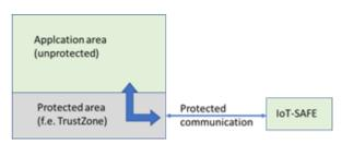
store all the main software parameters including the memory span and trusted signature. The IoT device must be able to secure communications with IoT SAFE. Many mainstream IoT devices can do so as they incorporate technologies, such as ARM TrustZone, where a protected area controls the boot process and the communication channel with IoT SAFE.
