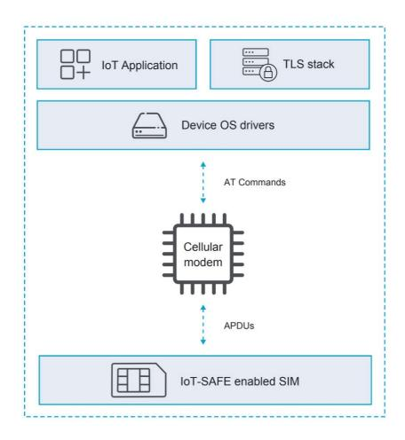
The most common way to access the IoT SAFE from the device is through the standard modem/module AT commands (described in [3GPP\_AT]) that provides a mean to forward messages to the SIM. Encapsulated within the AT+CSIM command, the IoT SAFE messages are exchanged directly between the SIM and the device application using an ISO7816 interface located in modem/module.
