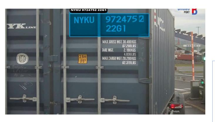
Use of **artificial vision technology** based on deep learning algorithms, applied to the real-time recognition of the signage of vehicles accessing for **automated access control.**
