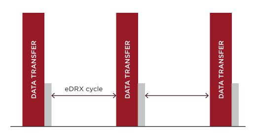
Between two consecutive PTW windows, the IoT device module or chipset enters a so-called "Sleep Mode" during which the receive path of the radio chipset is deactivated.
