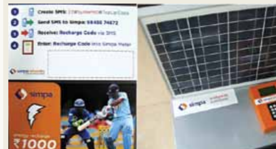
Figure 36: Simpa Networks Scratchcard and metering system
