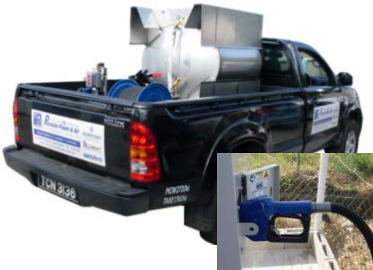
Custom Mobile Refueling System
