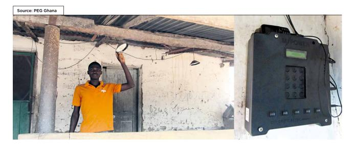
PEG agent with lights connected to SHS; SHS battery and control panel with keypad for manual code entry.
