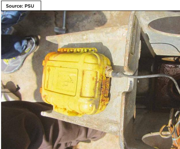
Testing pilot sensor after installation, hard carbon fibre casing on the outside to protect the antenna
